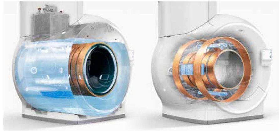
Classic magnet technology ~1,500 liters of liquid helium
