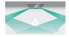
while one angled tweeter faces diagonally outwards. By introducing forward firing speakers without impacting Ambisound's surround sound capabilities, the system can now be much thinner.
