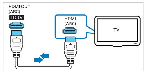
**1** Using a High Speed HDMI cable, connect the **HDMI OUT (ARC)** connector on this product to the **HDMI ARC** connector on the TV.
